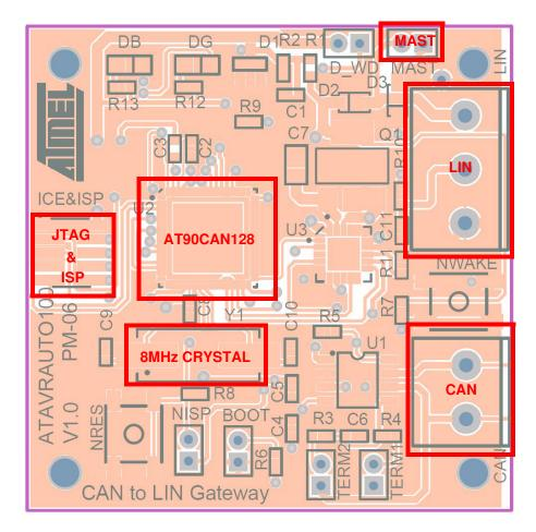
2.2 **Power Supply** The on-board power supply must be provided via the LIN connector. The ATAVRAUTO100 has been designed for operating voltage from 7V to +18V with typical voltage at 12V. The LIN transceiver ATA6621, connected to the LIN network, has an internal voltage regulator which outputs 5.0V ±3%. This voltage is used to power the AT90CAN128 device.
